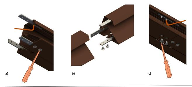
When the extensions are ready then the aluminum profile can be secured in place.
